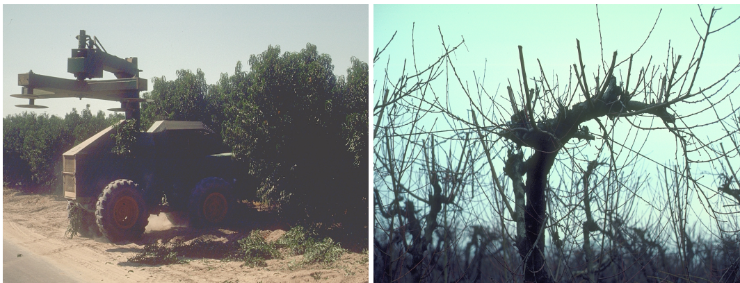
Fig. 5. A mechanical topping machine in a peach orchard and the types of heading cuts the machine leaves in the top of the tree.
